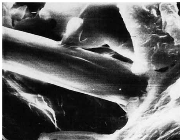
Figure 1 SEM view of the fiber/matrix interface of the COPPGF sample ( \times 3600 ).
