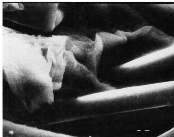
Figure 2 SEM view of the fiber/matrix interface of the PPGF sample ( \times 2400 ).
